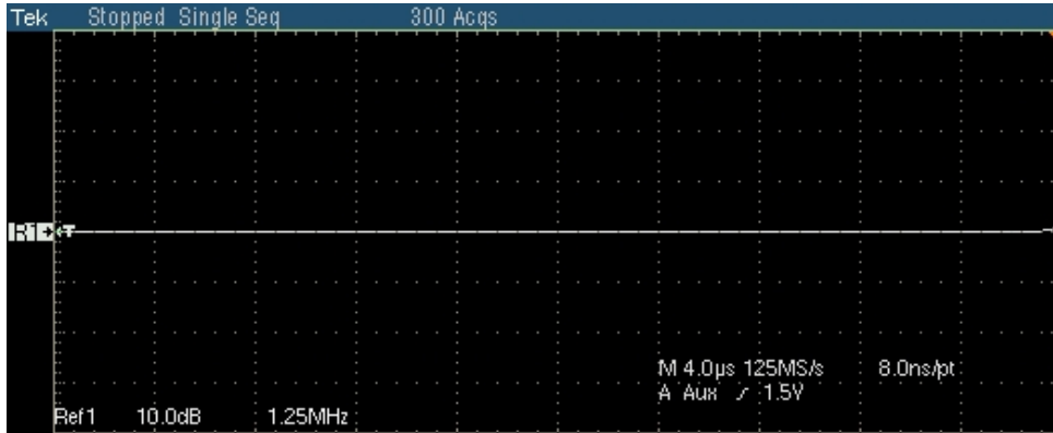
Figure 18-19: Waveform of 10BASE-T Return Loss Open calibration
