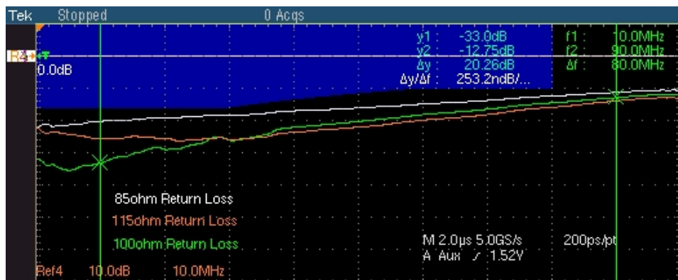
Figure 9-18: Waveform for 100BASE-TX Return Loss Transmitter
